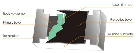
Fig 1. Construction of Chip-R WR02X
