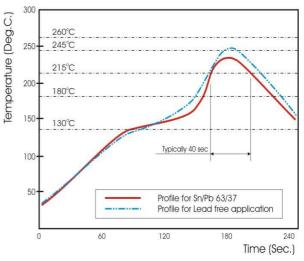
Fig 3. Infrared soldering profile for Chip Resistors WR02X(W)
